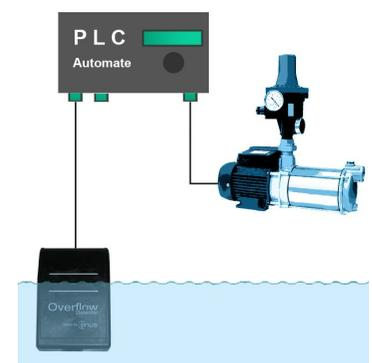
The CSC can also be connected to a Ijinus level sensor LNUV3, a data logger V3 Modbus and other PLC by Modbus connection
